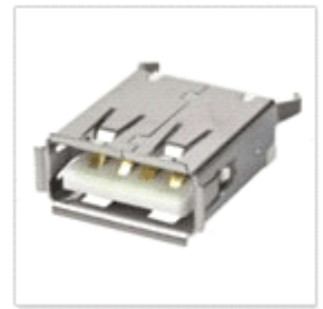
USB2-J USB AF, DIP Type Straight(180°)
